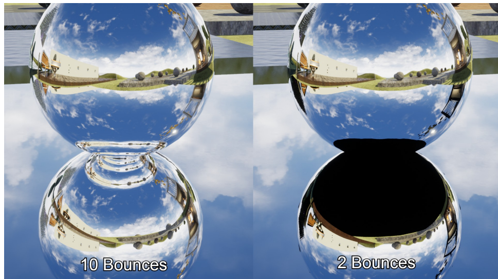
Figure 3.6: Small number of bounces between reflective objects can result in them appearing to be black.
