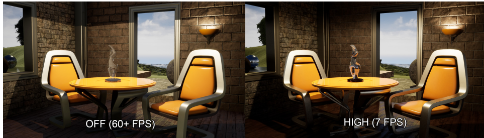
Figure 4.3: Turning all the available ray traced effects on decreases performance severely, even on the RTX 2070S.
