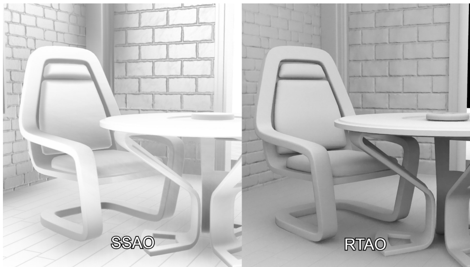
Figure 3.12: The difference between ray traced and standard ambient occlusion is more visible when we hide all but the ambient occlusion layer.
