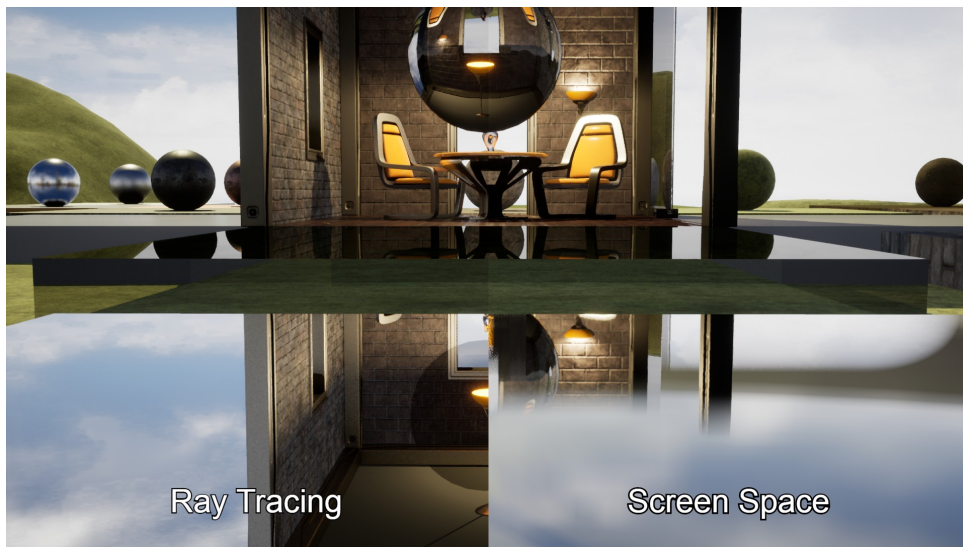
Figure 3.4: The screen space reflection on the right side of this image lacks the ability to reflect objects outside of the camera's view frustum.
